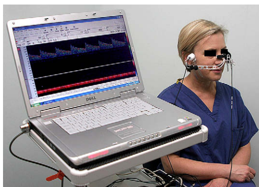
Fig. 1. PC-based transcranial Doppler system (Doppler-Box, Compumedics Germany GmbH, Hamburg, Germany) and probe fixation device suitable for perioperative use.
